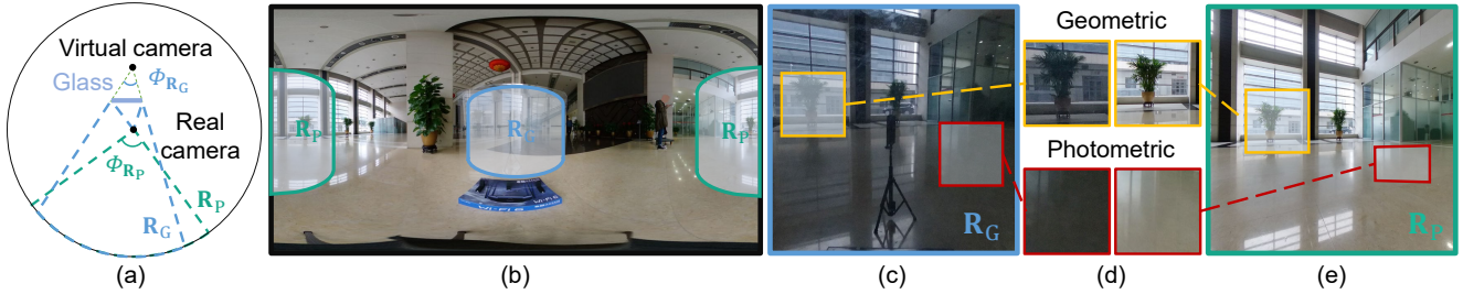
Figure 2. (a) Camera model of capturing a scene containing a glass plate by a panoramic camera. (b) Captured panoramic image. (c) Glass-reflected reflection image R_G , which is ‘captured’ by the virtual camera. (d) Illustration of the geometric and photometric misalignment. (e) Panoramic reflection scene R_P , which is captured by the real camera.
